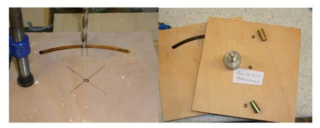
Drill the holes in the centre to suit your screw chuck and the outside holes in the **back plate only** to 8.5mm (21/64") for the threaded inserts. The top hat style inserts need to be screwed in from the back of the back plate and then if any of the insert protrudes through the plate filed flush with the plate.
