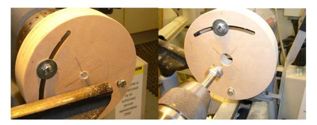
Fit to the chuck and drill or turn the 20mm jam chuck location hole.
