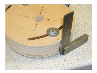
Mark the Zero Position and the 4mm fixing holes.
