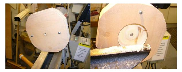
Turn a recess to suit your chuck on the back of the back plate. Beware of the protruding screws, always adjust the tool rest with the Lathe stationary and rotate by hand before starting the Lathe.
