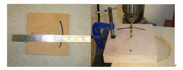
Mark out Drill position and transfer holes to the back plate.
