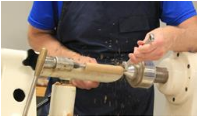
Using 5/8" WENCH AS GAUGE FOR DIAMETER SIZE
