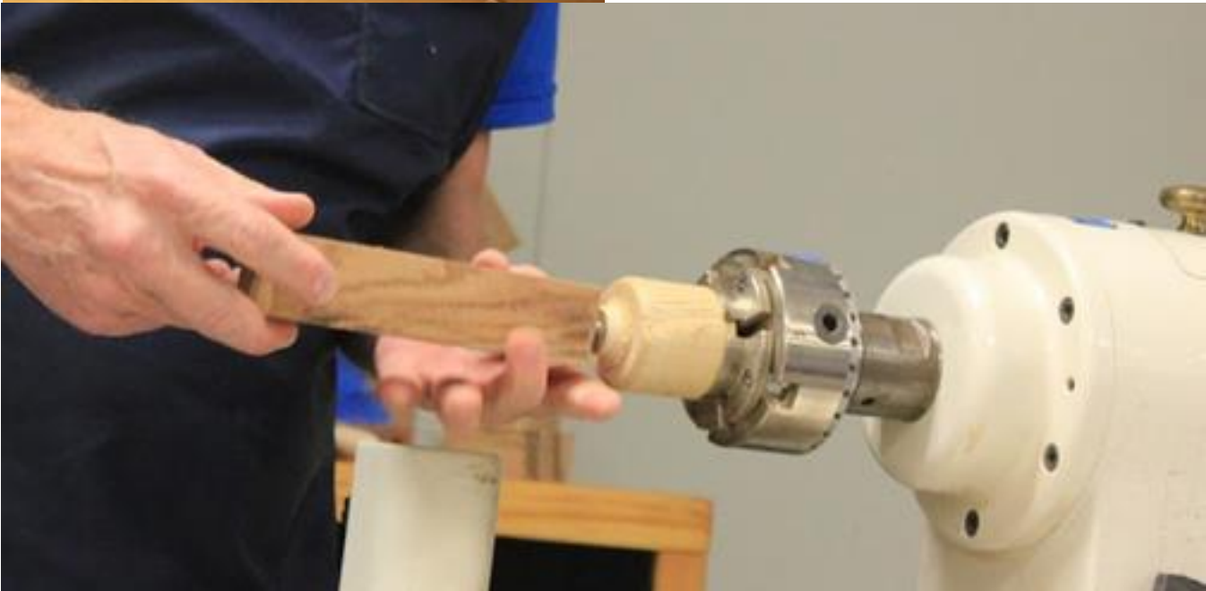
Jig for holding threaded insert handles
