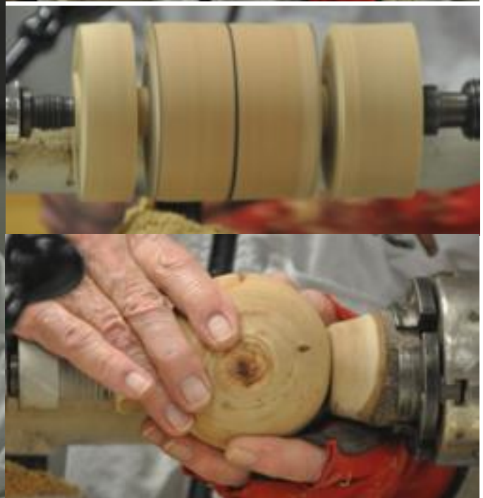
Mounting rough sphere between jamb chucks
