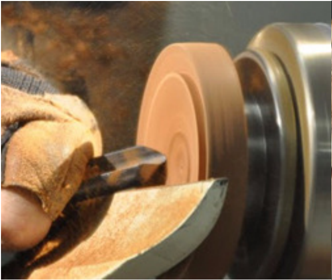
Bottom of the lid is made concaved
