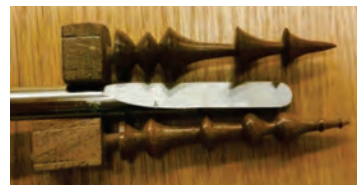
Top is 80 deg. Bottom is 35 deg. These are 1/2"x1/4" steel scrapers, top standard, and the bottom remade
