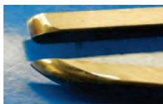
Top is 80 deg. Bottom is 35 deg. These are 1/2"x1/4" steel scrapers, top standard, and the bottom remade
