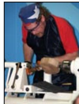
For this project, Craig uses dry stock, selecting contrasting or figured wood for the inlay if one is to be used. The blank for the vase is about 7" by 6" by 2" (or 2 1/2" if
