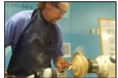
Since the piece should now be running balanced, you can remove the tailstock and begin the refining cuts. Start forming the wings, working from the outside in, then from the inside out. You may need to re-cut the bowl all the way from the bottom to the wing to get a smooth blending of curves.
