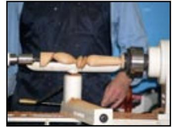
directions. While the piece is on these centers, the middle to bottom part of the candlestick is turned, though not
