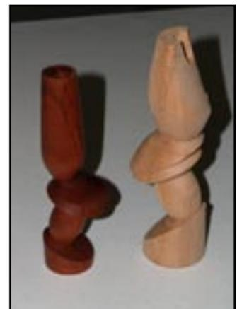
A dowel is placed in the candle hole at the top for the drive center. Using this set-up, the top is finish turned and the very bottom is squared up to the top and slightly hollowed.
