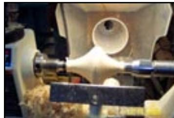
the center toward each end. The distance between the two end lines must be equal to the diameter. The piece is then parted down to tenons of about 5/8" diameter on each end. For safety's sake, he wraps both tenons and the center line with filament reinforced tape to ensure against the two pieces
