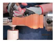
are going to put an insert (like a test tube) to hold water in the weed pot, then be sure to drill deeper than the insert. By doing this, you allow room for an air gap. Otherwise, you'll have difficulty getting the insert in due to the compressed air at the bottom of the hole.
