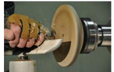
Then he turned a hollowed vessel using Easy Wood Tools three hollowing tools. One is nearly straight to hollow the center and slightly off-center part of the vessel, the second is slightly curved at the end to continue hollowing the sides of the vessel, and the third has a sharper curve at the end to turn out the top of the lip of the vessel. They all use a round cutter at the end.
