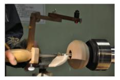
Jim also used the diamond point Easy Wood detailer tool on a spindle.
