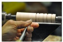
the middle of the 2 v-cuts. What the students learned is that each bead has a tiny flat spot, represented by the pencil line. The push cut starts on either side of the middle pencil line to form the bead. The push cut begins with the handle side down
