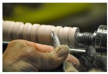
the handle up and curving the gouge face to the closed position. A cove cut is the opposite, it begins with the gouge closed, handle high, then lowered as the gouge face is opened. Finally,
