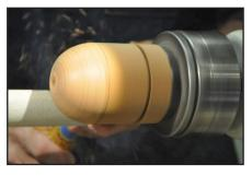
Next reverse the position of the piece into a jam chuck that you have hollowed out deeper than the curve of the ball. Your jam chuck should be sloped toward the sphere.
