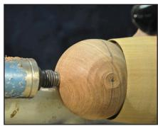
Flip the ball 180 degrees so the original mark that you cut (the one closest to the head of the lathe) is now facing toward the tail stock
