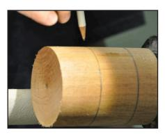
Starting out with a piece of wood approximately 2.5-3" rounded, draw two lines to third the piece. Mark the line closest to the chuck by cutting a mark with a thin parting tool.
