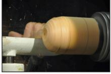
spaced toward the center (and end approximately the same distance to the curve) begin to form one side of the sphere.
