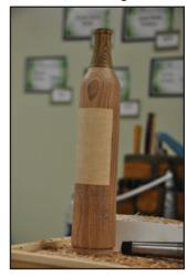
glued three boards together for the form, note the whiter board indicates where the label would be. Using two
