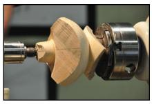
bowl and the legs converge. Use of detail gouge or a skew will simplify the process. It is easier to finish this area if the bowl and the legs form a wide vee. Making the legs have more arch keeps them away from the bowl and makes them easier to sand. For a variation, a cove or some other detail can be used in lieu of a vee where the bowl and base meet.
