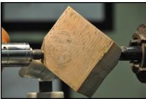
mounted on the lathe between those two centers, with the bottom of the bowl oriented to the tailstock. Using a bowl gouge, material is removed to form a tenon on the bottom. As material is removed, a triangular base will appear. This will become the foot of the bowl. The more material that is removed, the bigger the base will become. You need to remove enough
