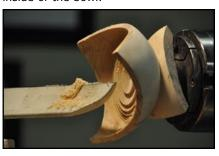
To finish the bottom of the base, chuck a 3" X 3" waste block and turn it to a convex shape a concave center, sort of like a donut. Reverse the bowl onto this waste block with a piece of leather between the two and bring the
