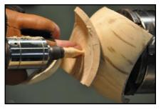
tailstock up to hold the bowl in place. Carefully remove the tenon and match the shape of the bottom of the legs to the shape of the top. Turn off as much of the tenon as you can, then remove the bowl, cut off the final nubbin and sand the bottom and apply the finish of your choice.
