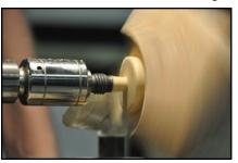
material to make a stable base as well as enough to create a tenon. The cuts should create a shallow bowl, which will give the legs an arched appearance. Finally, cut a tenon to fit your chuck. That tenon should be solid wood all the way around, with no flat spots and should be as small in diam-
