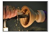
write the number on each ring to ensure accurate assembly. The piece is glued up in a similar manner to the first two methods. Instead of gluing to the face plate, the first ring is held in place with small pieces of doublestick tape. If Mack is making a hollow form, he glues it up and turns it in two pieces to allow him to hollow the insides before he glues the two halves together to form the finished vessel.
