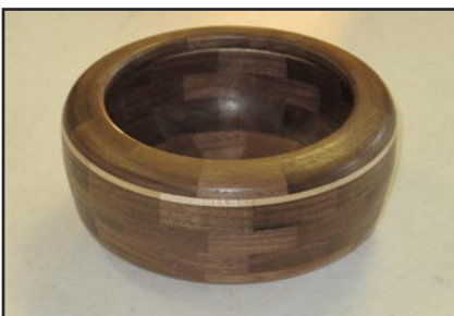
H.O. Evans' "A Thing" segmented piece with captured ring. HO said it was pretty difficult to "capture" the ring.
