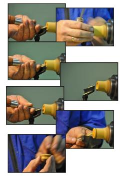
Next he SLOWLY turns the ogee on the bottom of the base to the same dimensions matching the lids and mortise. This allows him to be ready for the next lid/base combination. The most amazing part of this adventure is the number of boxes that he can turn in the stump of wood! Since all dimensions match, the combinations of tops and bottoms are limitless. We appreciate Steve's trip to Austin and wish him a safe trip back to Michigan after his Texas Winter vacation.
