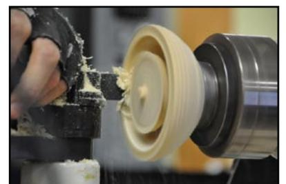
finished the first coring, he took it out, chucked it between centers and turned a tenon on it and cored a second bowl. Normally, he would use a much bigger blank and wind up with four or five rough-turned bowls to dry in bags of chips for later finish turning.
