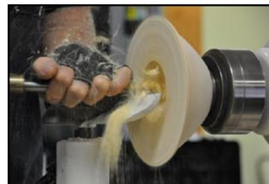
paper bag full of chips before turning them to final shape.) The piece was then reversed, with the tailstock providing the pressure to hold it against the chuck so that he could turn off all of the tenon except for a nub, which he then carves or sands off. (If you haven't turned away the hole made by
