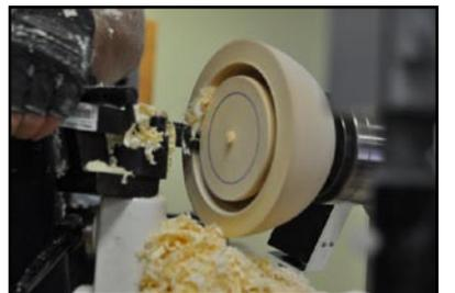
a blank that he had already prepared. That blank was chucked, the coring lines were marked on it and the process begun. He chose the proper chisel and began cutting out the first core, taking care to withdraw the tool frequently to clear chips. When he had
