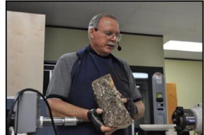
placed in the chuck and the inside turned. He used a drill bit to establish depth and kept checking wall thickness as he went along, emphasizing the
