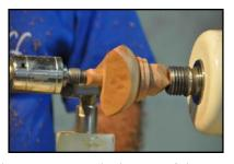
his attention to the bottom of the box, turning it into a spherical shape, but leaving about 1/4" of the corners unturned, before turning a tenon on the bottom.
