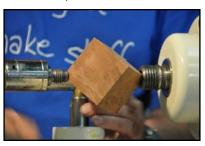
the cup of the live center with the point removed, carefully adjusting the position until the turning corners of the cube are perfectly aligned.
