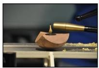
tenon is turned first, then an on-center tenon is turned on the bottom half of the first tenon. The end of the finial stock is turned round to fit precisely in the hole in the jam chuck. He turns the off-center section of the finial first, then turns the base of the finial and the tenon to fit the hole in the lid, then parts it off.
