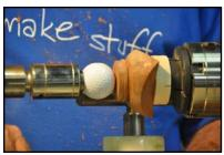
snugly fits in the hole and that has its face turned to a convex curve that fits the concave top. The piece is jammed on and held in place by a golf ball fitted to the live center and the spherical shape of the bottom is completed.
