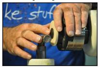
jaws on the wooden collet chuck holds the lid snugly while it is finished and a hole is drilled to fit a finial.
