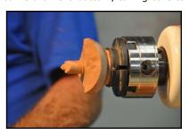
get a smooth curve and to stop the turning precisely as the curve of the top and the curve of the bottom meet at the points of the corners.
