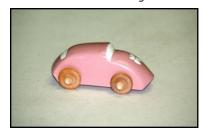
wheels and axles from Woodworks (800.722.0311), Part No. TW-1003 for the wheels and Part No. AP-1010 for the axle pegs. The axle pegs will have to be shortened about 1/4" to 1/2"
