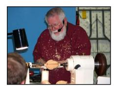
sanded on the lathe, sanding first with the lathe going forward, then with it reversed, or if you lathe won't reverse, by reversing and rechucking the piece.
