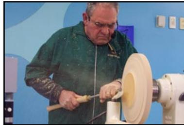
the center hole and trued it up. After drawing a 3" radius circle, he shaped the base of the platter outside the circle. He then drew 1" and 1 3/8"
