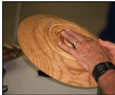
The screw chuck was then mounted in the first circumference hole 1 5/8" and 2/18" circles were drawn around this new center on the bottom of the platter. A 1/4" deep channel was turned between these two circles, sanded and textured. The same procedure is followed for holes 2 and 3.
