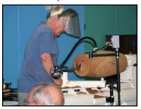
shape and hollow it. He then mounted a prepared blank on the headstock and proceed to show us his hollowing technique. Although he didn't use it
