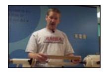
For the spurtle (stirrer), Rusty starts with a blank approximately one inch square and about thirteen inches long. In this spindle turning project, he uses
