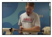
the skew is used to lay out the bead that will be the feature of the design of the piece. Rusty then begins to shape the spurtle with the spindle gouge, using his thumb on top of the tool and two fingers underneath and around the tool rest to support it. When he is satisfied with the general
