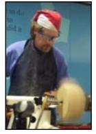
center. Rub the bevel, but don't push the tool into the wood. When the top is flat, cut a tenon on what will be the top of the bowl.
