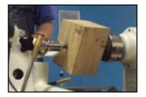
to cut one straight side on the blank, then place that side against the miter fence to cut the next side, proceeding until the blank is complete.
