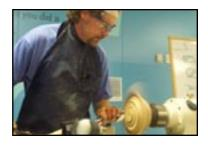
Since the piece should now be running balanced, you can remove the tailstock and begin the refining cuts. Start forming the wings, working from the outside in, then from the inside out. You may need to re-cut the bowl all the way from the bottom to the wing to get a smooth blending of curves.
