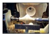
the center toward each end. The distance between the two end lines must be equal to the diameter. The piece is then parted down to tenons of about 5/8" diameter on each end. For safety's sake, he wraps both tenons and the center line with filament reinforced tape to ensure against the two pieces
