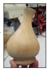
a less aggressive burr or aggressive sandpaper, then to a softer pad with hook-and-loop paper up to 120 grit, finally switching to a super soft pad for the finer grits.
