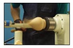
With these two points set, you can begin to waste away to connect the two. Craig uses a scraper with a very light touch to shape up the curve.
