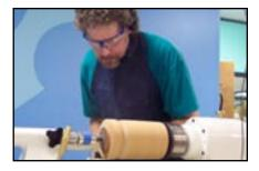
hole into the bottom, going as far into the neck as possible. He hollows with a Jamieson rig, but uses Kelton hollowing tools. He hollowed as far into the neck as possible, checking against the sketched neck shape on the outside of the top.
