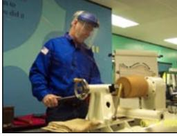
removed the hollowing rig and began to work down the stem, shaping and cleaning up as he went, so that he wouldn't need to use a steady rest.
